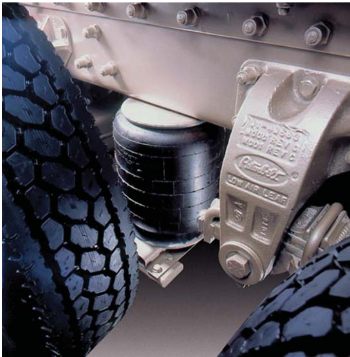
Air springs are highly engineered elastomeric bellows with specially designed metal end closures that contain a column of compressed air. The bellow itself is made of calendered rubber and high-strength, fabric-reinforced rubber.
